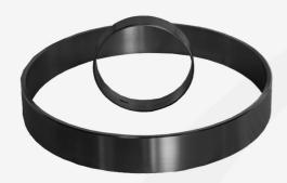
These are available in wide range suitable for light, medium and heavy duty application. Anti-Polishing Ring are 'cast-in fit', force (press) fit or slip fit. The interference between its outer diameter and bore-hole walls depends on fit-type from 0.050 to 0.100 mm. Anti-Polishing Ring, made of grey cast-iron, ought to have desired casting and machining qualities, viz. strength, toughness, hardness and wear resistance.
